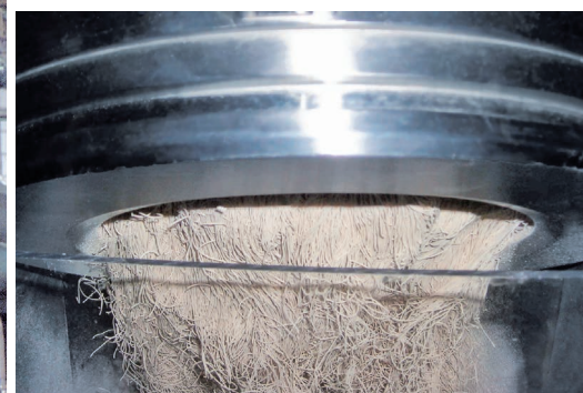
Filtered yeast passes through an extruder
