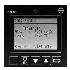
The necessary process values (such as ethanol concentration, temperature and sensor resistance) are locally displayed at the instrument and, for the purpose of process control, converted to a standard current signal and two limit relay contacts which can be used as input signal for any process control system or for visualization and/or documentation.
